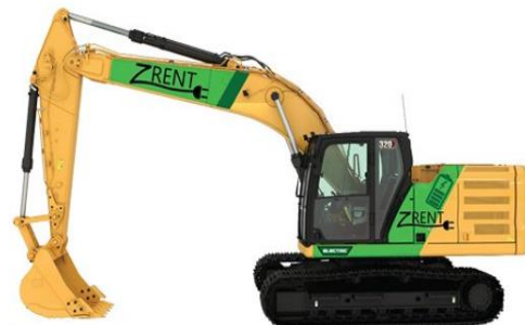
CAT 320 Z-LINE (Gravemaskin (EL)) Batteri – 300 kWh – max. 120 kW
