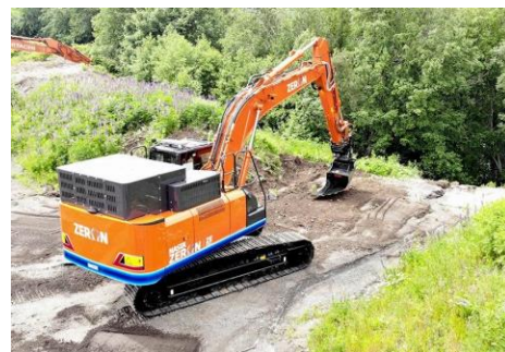
Hitachi Zeron ZE210 (Gravemaskin (EL)) Batteri – 300 kWh – max. 128 kW
