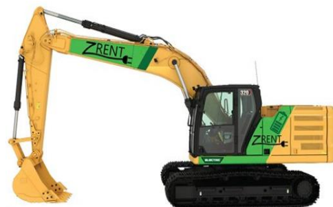
CAT 320 Z-LINE (Gravemaskin (EL)) Batteri – 300 kWh – max. 120 kW
